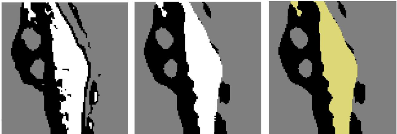
Figure 4. Raw classification > Modal filter applied > Vectorised with GRASS smoothing algorithm. Beach is shown in white (raster classification cells) and yellow (final 'Beach Area' polygon).
